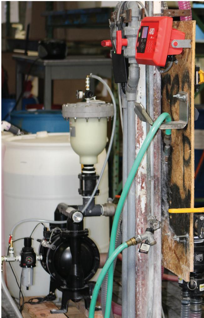
day and reduces the tedium of having to stand and watch the tanks fill to make sure nothing goes wrong. If the Controller senses a problem in pressure or process, it sounds an alarm.
